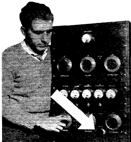
M. B. Kahn of the Collins Radio Company inspecting a Collins Transmitter furnished Byrd Antarctic Expedition. Arrow points to Bliley Mounted Crystal which is standard equipment on the set.
